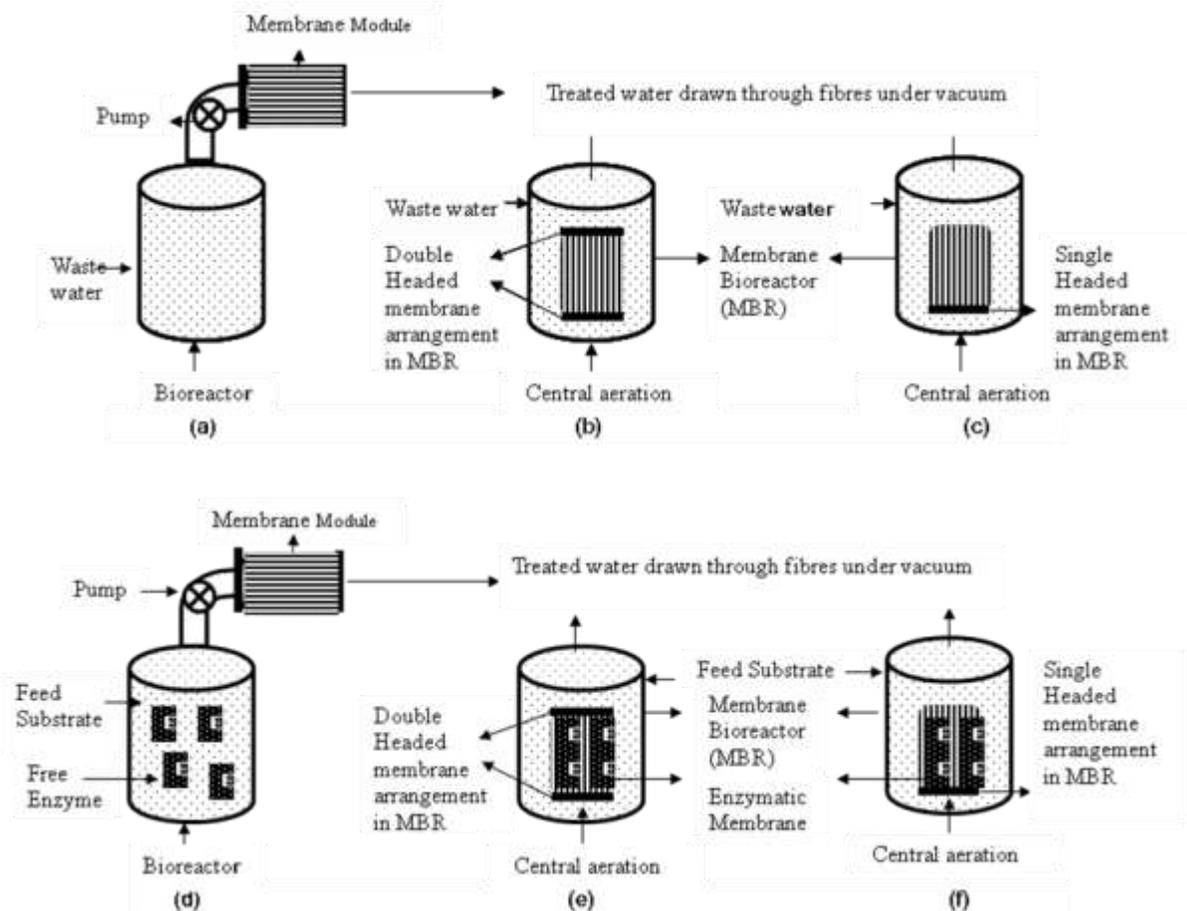
**Figure 5.3:** Different arrangements of membrane bioreactors (MBRs) and enzymatic membrane bioreactors (EMBRs)
